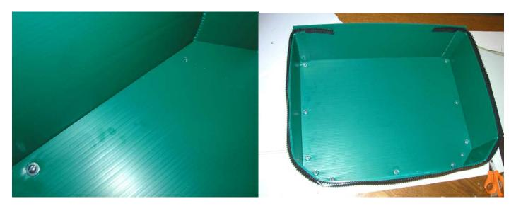
23. Line up the back edge of the box with the back tabs and drill, from the outside (it's easier), two holes. These holes should be placed at the ends of the tab (as is reasonable). Set T-nuts and screws in these holes to hold together. See figure.
