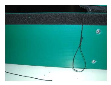
31. You will now be making a prussic knot to tighten the zipper ends together. Using the figure as a guide, follow the loose line around and out of the loop. The finger you see is holding the loose end of the line, and the loop is originating from the right side. Tighten the knot down, open up and slide it to tighten the line between the zippers. See figure.
