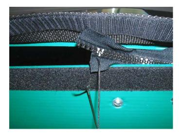
30. Tie a loop in one of the lines, about 3-4" in length. Cut of the excess. See figure.
