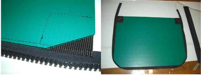
17. Pre assemble the lid onto the sides. Use only one slider to do this. This will allow you to see which teeth from the lid should line up with which teeth from the sides. Assemble the two pieces until the lid is *centered* on the sides, and then mark with a silver sharpie on both halves of the zipper, both ends of
