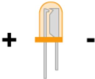
Looking at the 'internals' through the side of the LED the negative (-ve) or cathode side is sometimes wider than the positive (+ve) or anode side.
