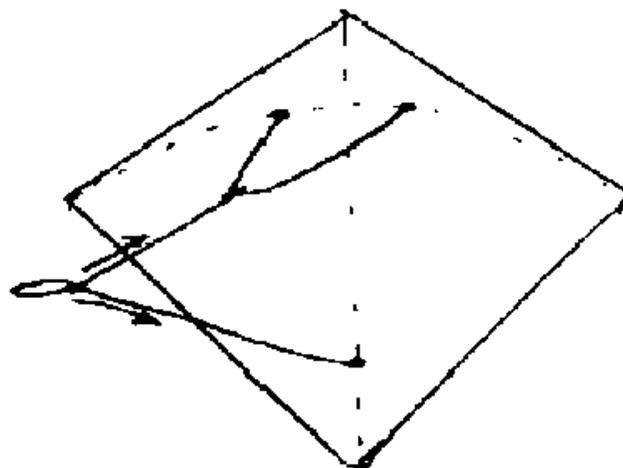
Position the tow connection loop at a point along the lower bridle leg that allows the kite to hang at a slight angle, nose up/tail down.
