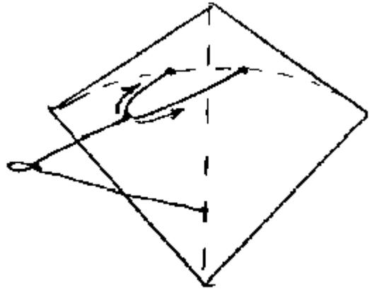
You adjust for it by moving the lower bridle leg's larkshead knot along the upper bridle yoke until the kite flies straight when strong tension is applied to the flying line. When the right/left bridle adjustment is correctly positioned, the kite won't have any tendency to veer or constantly turn to one side or the other!
