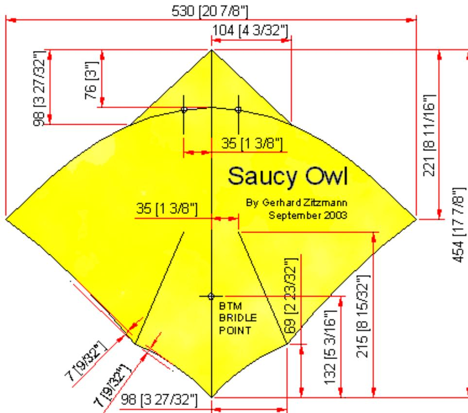
The saucy owl is a big and precise flyer for experts or also for beginner. The plan is special for low wind conditions. For very low wind i build it with 0.05 inch Carbon bow, then the kite fly slow and so it is also good for learning to fly with fighterkites. When you build it with 0.06 inch Carbonbow the kite shows his true self.... The spine i made from bamboo and the battens are 0.03 inch carbon. For the sail i use Orcon or Polypropylene Film.
