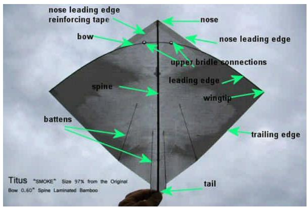
This is the back side of a buka showing names of various parts of the kite and the following photo shows the names of the parts of a 3-point bridle typically used on a buka.
