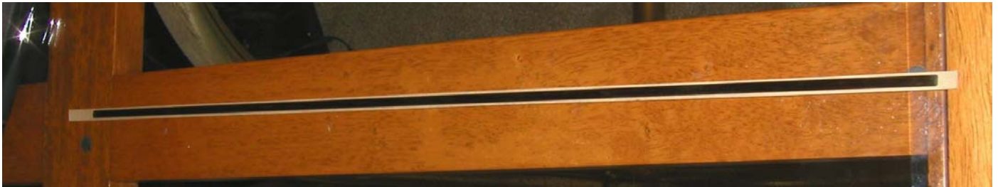
Figure 7: Flat carbon spine applied to center of 1/4" tape
