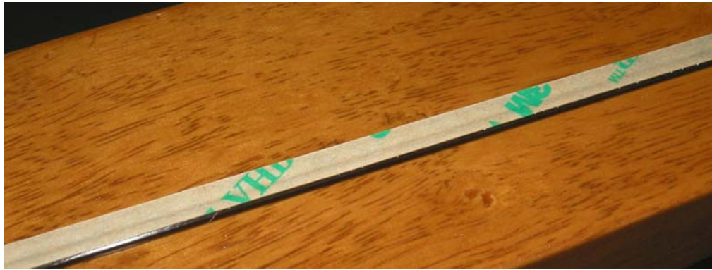
Figure 10: The finished spine with adhesive, ready for applying to sail.
