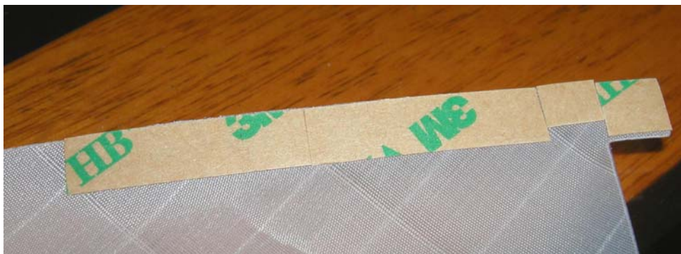
Figure 5: Small pieces of tape on the leading edge. Keep them as close as possible to the edge of the fabric. Close!!
