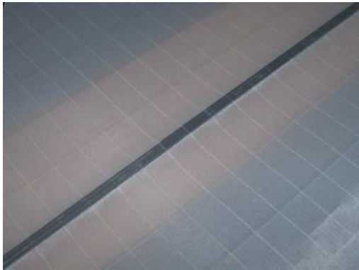
Figure 15: Fully adhered spine to sail.
