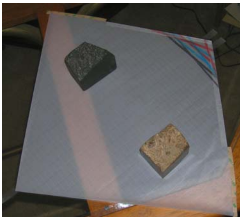
Figure 12: Sail is drawn out firmly flat using two pieces of tape at the nose, one at the tail, and two fabric weights.
