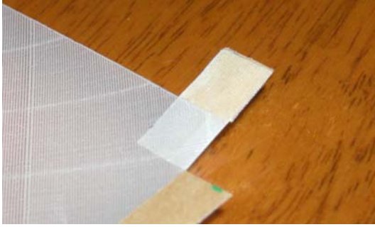
Figure 19: The piece now folded over and adhered to the sail.
