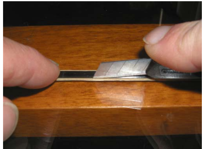
Figure 9: Cutting the excess tape off the spine.
