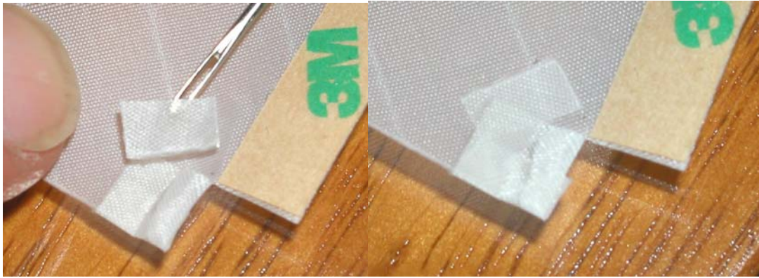
Figure 23: Application of reinforcement to spar pocket.
