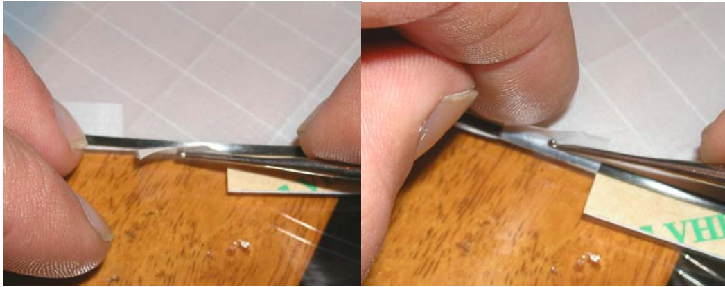
Figure 29: Wrapping the roll over around the bow spar.
