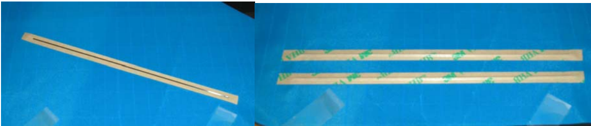
Figure 34: Batten applied to tape, then applied to fabric creating sandwich of fabric, batten, and adhesive.
