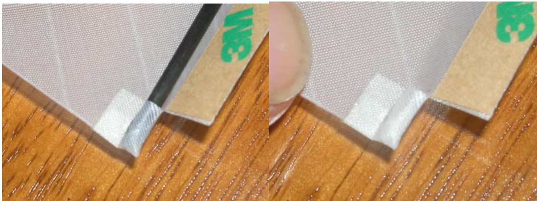
Figure 22: Sizing the spar pocket with rounded graphite, leaving a crease as to where it will be.
