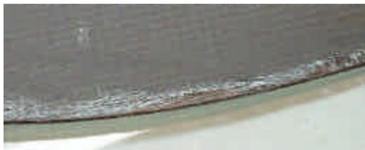
The photo above on the left shows cutting off excess hem material. You can see in the photo on the right the extra glue on the kite skin that wasn't needed. Dust the exposed glue with cornstarch to remove the stickiness.
