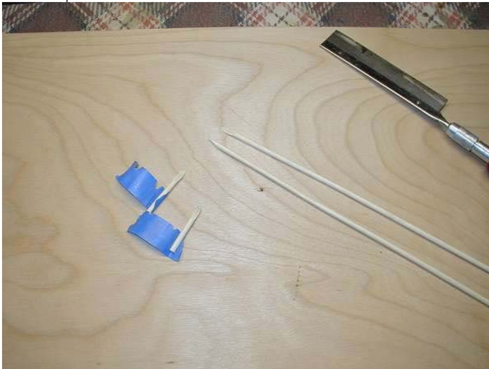
I use Titebond glue. Rub each scarfed end into the glue - this presses the glue deep into the 'boo fiber. Rub it in good 'til it's kinda sticky ...
