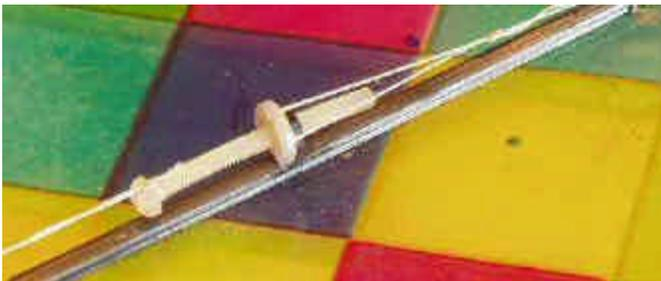
This is a simplified version of Chuck's nylon nut and bolt idea; I just drilled holes in the head of the bolt and into a nylon washer for the line. I have also drilled holes into the bolt like Chuck did. Both work.
