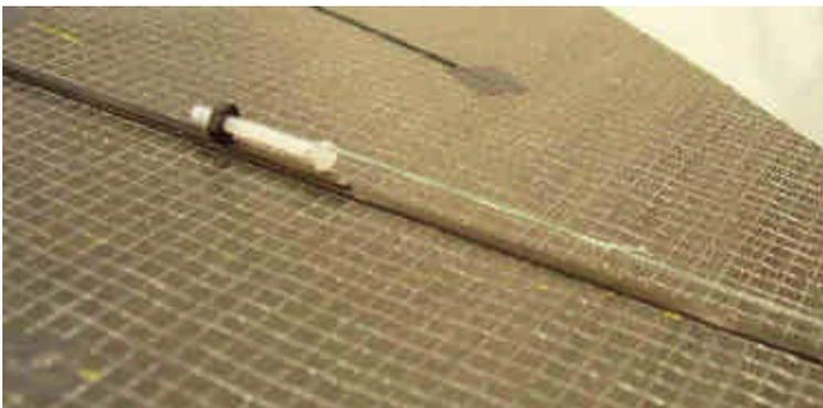
I experimented with modifying Chuck's nylon nut and bolt arrangement. I drilled a hole through the flat carbon spine into the edge face of one of the nut facets, then inserted a short piece of 0.03" diameter carbon rod and glued it. The short rod acts like a post to help hold the nut onto the spine. Glue alone would probably not be sufficient because the tension needed to create the bend in a spine can be substantial.
