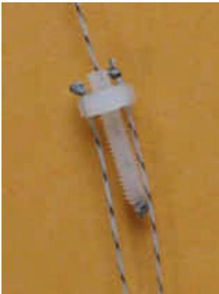
Chuck Lund thought of the 'brilliant' idea of using a nylon nut and bolt as a spine adjuster mechanism. Drilling small holes in the head of the bolt and the nut to thread the tension line through is all that is needed. It works very well. As you can see Chuck drilled through the center of the bolt and nut to attach the lines.
